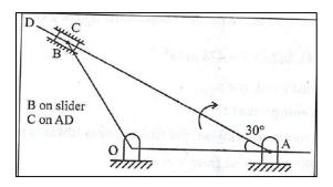
6. The crank OA of a slider crank mechanism shown rotates uniformly at 20 rpm counter clockwise. The dimensions of different links are: OA=300 mm; AB =1200 mm; BC = 450 mm; CD = 450 mm; determine the linear acceleration of sliders B and D.
