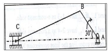
9. Locate all the instantaneous centers for the crossed four bar mechanism shown, the dimension of various link are: AB = 55 mm; BD = 80 mm; AC = 60 mm and CD = 65 mm. Find the angular velocities of the link AB and BD if the crank CA rotates at 100 r.p.m in the counter clockwise direction.
