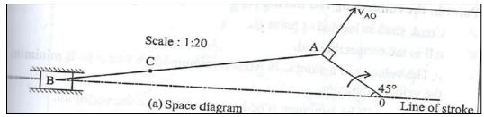
5. A single cylinder rotary engine is shown below. OA is the fixed link, 200 mm long. OB is the connecting rod and is 520 mm long. The line of stroke is along AD and at the instant is inclined at 30<sup>0</sup>. The body of the engine consisting of cylinder rotates at a uniform speed of 400 rpm, about fixed centre A. Determine the acceleration of the slider B and angular acceleration of connecting rod. [AU, April/ May 2015]
