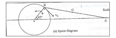
4. The crank and connecting rod of a theoretical steam engine are 0.5 m and 2 m respectively. The crank makes 180 rpm in the clockwise direction. When it has turned 45<sup>0</sup> from the inner dead centre position, determine: [i] velocity of piston [ii] angular velocity of connecting rod [iii] position and linear velocity of any point on the connecting rod which has the least velocity relative to crank shaft. [AU, April/ May 2015]
